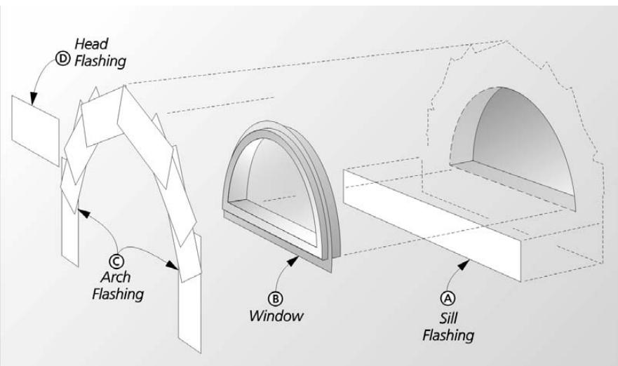
**Note:** Each opening should be treated independent of the others. Starting at the lower windows, work toward the top. The installation of all windows must follow the proper sequence of installation, as opposed to trying to flash all of the windows at once to save time, save material, or make the job easier. Fortifiber recommends the use of a well integrated weather-resistant barrier with all of its flashing systems.
