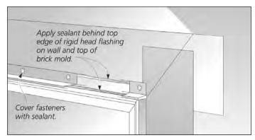
Prior to installing the rigid head flashing apply a 3/8" bead of sealant to the top of brick mold. Then place sealant on the top edge (interior side) of rigid head flashing. Place head flashing over brick mold and fasten with galvanized nails or screws. Apply sealant over these fasteners.
