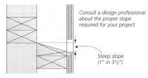
For proper drainage the exterior wall sill must be sloped. The example above shows a steep slope (1" inch in 3½"). This slope can be created by ripping dimensional lumber. Please consult a design professional about the proper slope required for your project
