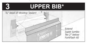
Before installing bib, place a 3/8" bead of **Moistop Sealant** as shown above. Then cut the **Super Jumbo Tex** to the width of the exterior wall rough opening. The height goes from flush with the interior wall sill and extends 2" inches
