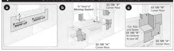
The Starter bib is made from a 12" inch piece of **Moistop neXT** that is attached to the exterior wall 3" above the bottom of the sloped sill. Remove the section of **Moistop neXT** that is between the exterior jambs and sill by cutting flush with a sharp utility knife, see1a.
