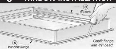
Before installing the window **(C)**, apply a continuous 3/8" bead of **Moistop Sealant** to the perimeter of the rough opening or to the backside of the mounting flange **(D)** of the window. Install the window according to the window manufacturer's instructions.
