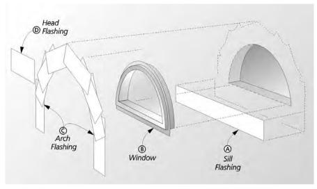
**Note:** Each opening should be treated independent of the others. Starting at the lower windows, work toward the top. The installation of all windows must follow the proper sequence of installation, as opposed to trying to flash all of the windows at once to save time, save material, or make the job easier. Fortifiber recommends the use of a well integrated weather-resistive barrier with all of its flashing systems.
