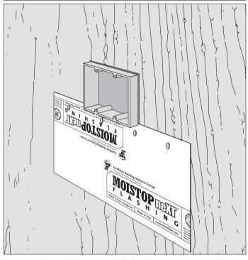
Install minimum 9" **Moistop neXT** flashing as bib under utility box. This flashing should be a minimum 8" wider than the utility box.
