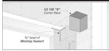
Apply a 3/8" bead of **Moistop Sealant** as shown above. Firmly press the **GS 100 "B"** piece into the sealant. Trim and fold this piece as shown at right. Then fasten in place.
