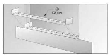
Place the sill pan with sides upturned in the rough opening. The leading edge of the sill pan must be aligned with the front of the rough opening.
