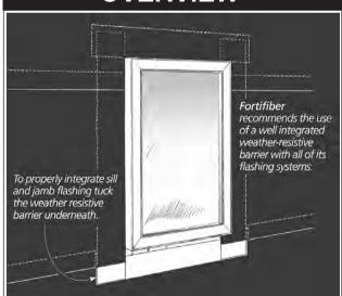
This recommendation refers to the most common types of windows used (surface mounted). For other types of frames, special attention should be paid to the window manufacturer's instructions.
