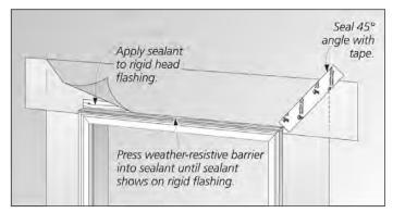
Place a 3/8" bead sealant along the lower portion of the upturned leg of the rigid flashing. This will allow the weather-resistive barrier to be applied in sealant. Finally, allow the flap of the weather-resistive barrier to lay flat over the sealant and rigid head flashing. Press flap into sealant and apply a new piece of sheathing tape over the entire diagonal cut made in the weather resistive barrier and press firmly in place.
