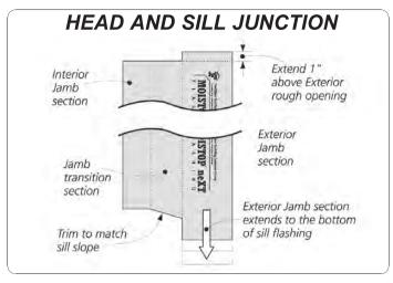
Moistop neXT is used for Jamb flashing. This piece starts 1" inch above the top of the exterior wall rough opening and extends even with the bottom of lowest piece of sill flashing. The detail above shows how to notch the jamb piece properly at the head and sill. Once the jamb flashing is in place, trim the sill flashing flush.
