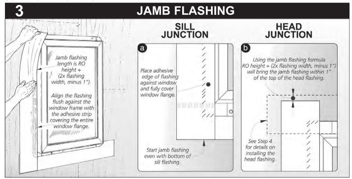
Prior to installing the jamb flashing, wipe the window jamb flange and exterior walls with a clean rag to ensure proper adhesion. Cut the jamb flashing to the height of the rough opening + 2x the width of the flashing, **minus 1"** (see 3a and 3b). Remove the release paper and place the jamb
