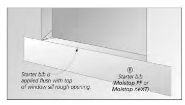
Cut the starter bib to the width of the rough opening plus twice the jamb flashing width, minus 1". Attach the starter bib flush along the bottom of the rough opening.
