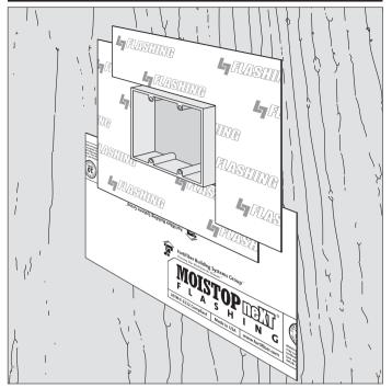
Install upper/side piece of **L7 Flashing** into sealant and over previous piece.
