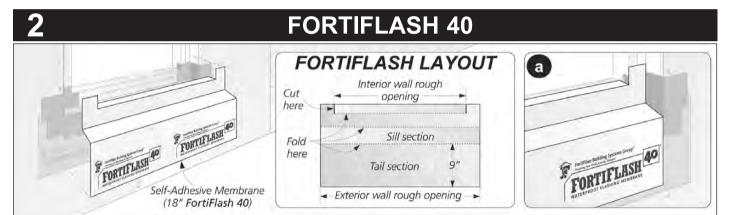
A piece of 18"-wide **FortiFlash 40** is used for the next layer of protection. To prevent wrinkles, or airpockets while installing this piece of self-adhesive flashing the following sequence is strongly recommended.
