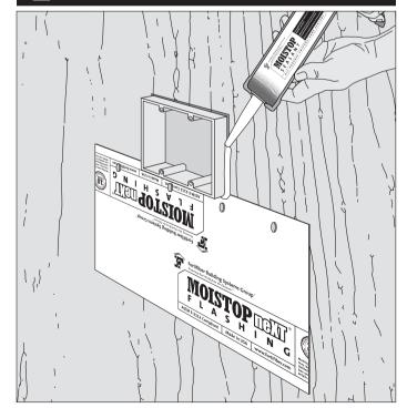
Fill any gap between sheathing and utility box using appropriate method. Apply a minimum %" bead of **Moistop Sealant** around utility box.
