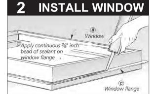
Before installing the window, apply a continuous <sup>3</sup>/<sub>8</sub>" bead of **Moistop Sealant** to the backside (interior) of the mounting flange. Install the window according to the window manufacturer's instructions.
