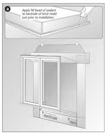
Before installing the door or window, apply a 3/8" continuous bead of Moistop Sealant (9a) to the backside (interior) of the brickmold. Install the window or door according to the manufacturer's instructions.
