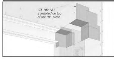
Press the **GS 100 "A"** piece into place on top of the "B" piece installed in Step 6. Fasten as shown at right.
