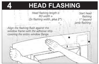
Wipe the head flange, jamb flashing and sheathing with a clean rag. Cut the head flashing to twice the width of the rough opening + 2x the width of the flashing **plus 2**". Install the head flashing by pressing firmly in place in one direction to prevent voids.
