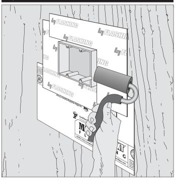
Use a J-roller to remove wrinkles and adhere flashing to the substrate.
