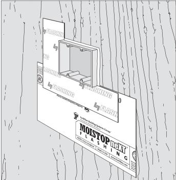
Install bottom/side piece of L7 Flashing into sealant.
