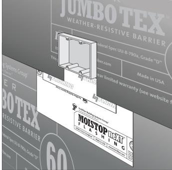
Install water-resistive barrier around box and integrate under **Moistop neXT** flashing.
