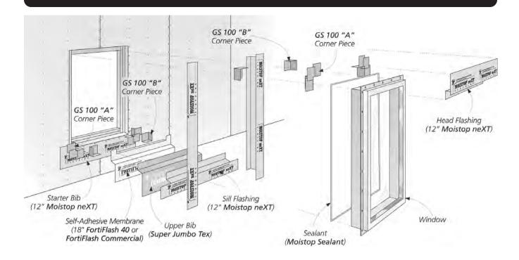
This installation guide adresses the proper flashing of a window that is contained in a recessed wall system built using a double 2 x 4 wall. Also the window is installed and flashed before the weather-resistive barrier is applied. For other wall configurations consult a design professional. **Note:** It is the responsibility of the installer and General Contractor to consult with the manufacturer on how these instructions apply to the
