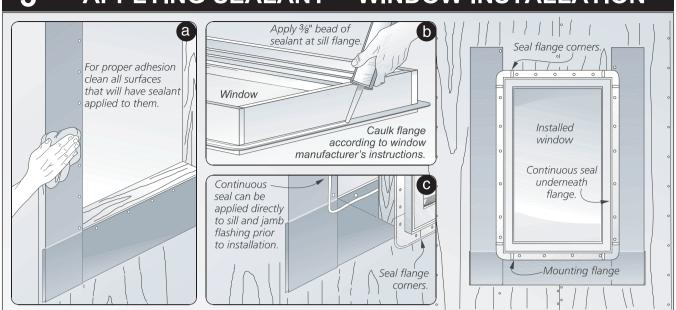
To insure the proper adhesion, wipe the window flange, sill and jamb flashing with a clean rag before applying **Moistop® Sealant (3a)**. Prior to installing the window, apply a continuous 3/8" bead of **Moistop Sealant** to the backside (interior) of the
