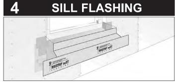
Moistop neXT is used as a protective course for sill flashing. It is fastened flush with the top of the interior sill, covers the exterior sill, and extends to the edge of the jamb flashing installed in Step 5. Since the length of jamb flashing can vary, run the sill flashing long and trim once jamb flashing is installed.
