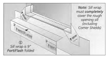
Cut 9" **FortiFlash** to the width of the rough opening. Align back edge of **FortiFlash** to the marked fold line of the sill pan and fold over the front of the bib.
