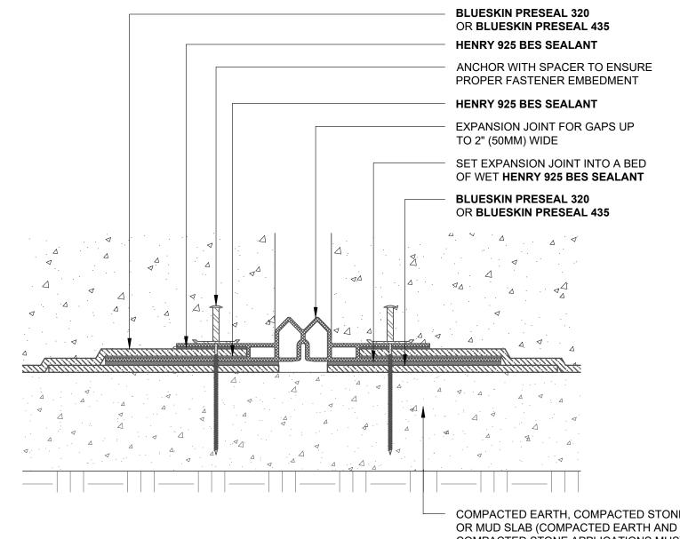
OR MUD SLAB (COMPACTED EARTH AND COMPACTED STONE APPLICATIONS MUS USE BLUESKIN PRESEAL 435)
