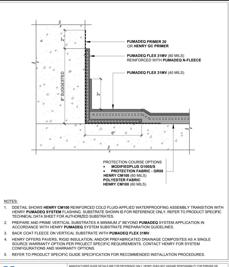
MANUFACTURER GUIDE DETAILS ARE FOR REFERENCE ONLY. HENRY DOES NOT ASSUME RESPONSIBILITY FOR ERRORS OF DEVIATIONS IN DESIGN OR ENGINEERING. PROJECT SPECIFIC VERIFICATION IS RECOMMENDED PRIOR TO INSTALLATION. HENRY CM100 AND PUMADEQ SYSTEM TIE IN
