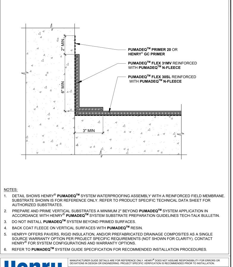
PUMADEQ<sup>™</sup> SYSTEM - WATERPROOFING ASSEMBLY
