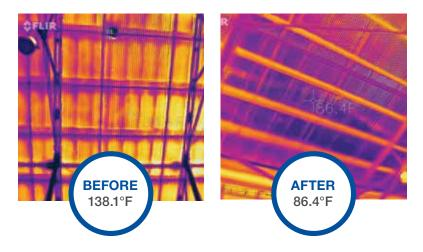
An installed SPF and coating roof system can lower the interior temperature of a metal roof by 20°F to 50°F compared to a typical existing metal roofing system. A cooler roof provides energy savings, especially in warm climates. PremiR+ EVO is a proven system engineered to reduce energy bills, extend roof service life, and improve occupant comfort.
